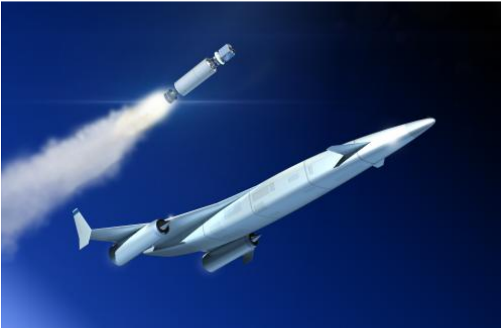
Artist's impression of the release of an upper-stage from a next-generation SABRE-powered reusable launch vehicle. The development of the SABRE technology will enable low-cost, high-cadence space access. (Reaction Engines image)
